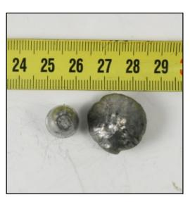
.45 cal Pedersoli Minié bullet fired from a Pedersoli Mortimer Whitworth rifle. E0=2720 J, bullet recovered from ballistic gelatine
